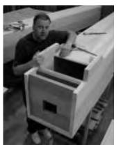
feet deep. The supporting wall behind is 120 feet tall. Meanwhile, back in the shop, the windchests, swell boxes, reservoirs and the terraced console are all under construction. At left, John Ourensma prevoices the 32' Bourdon, which was built here in Lake City.
