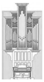
Dobson Op. 77 (II/21), for United Lutheran Church in Red Wing, Minn., was installed in February and March, 2001. The Swell and Great divisions are in a free standing case of oak with a detached, mechanical console placed in front for ease of choir direction. The pedal division has electric action and is located in the old organ chamber directly behind.
